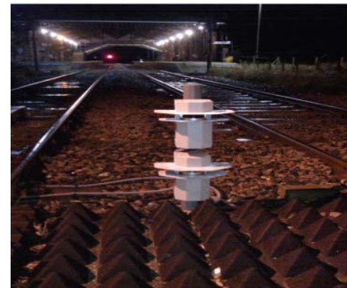
MCB-OD Radar (top), Lidar (bottom left) and the area of obstacle detection provided
